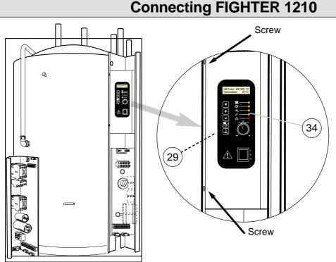
Open the top cabinet cover by loosening the screws on the front. Loosen the screws holding the control computer (34) and release the piece from heat pump. The relay card (29) is now easily accessible to connect the sensor (86) on terminal block (30). See the wiring diagram on the first page for connection details.
