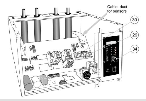
Loosen the screws holding the front panel and lift it off so the electrical connection area is accessible. The relay card (29) is now easily accessible to connect the sensor (86) on terminal block (30). See the wiring diagram on the first page for connection details.
