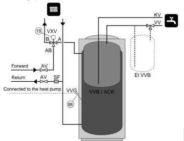
In order to reach the maximum hot water temperature, hot water charging is stopped by the operating pressure switch on the heat pump. The water heater is equipped with the requisite safety equipment.
