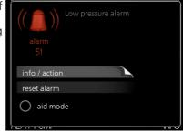
remedy itself. In the display, by turning the control knob and pressing the OK button, you can see the type of alarm it is and reset it. You can also choose to set the heat pump to aid mode.
