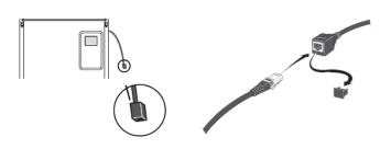
3. Insert the Ethernet cable to the cable on the backside of the system as seen on the picture above. If you have upgraded your system with NIBE Uplink you can attach the cable directly to the display as shown below.
