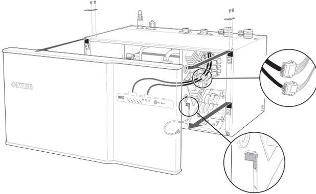
1. Remove the screws in the top panel.
