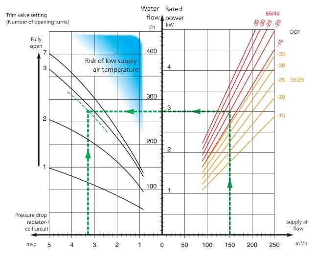
The delivered output in the diagram is calculated when dimensioning the heating system 55/45°C respective 35/25°C (underfloor heating).
