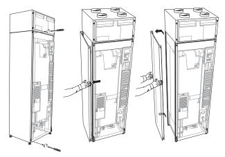
The side covers can be removed to facilitate the installation.
