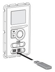
The display unit is equipped with a USB socket that can be used to update the software, save logged information and handle the settings in F470.
