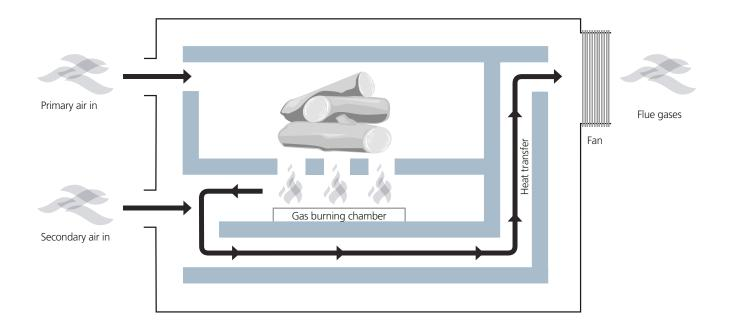
In a NIBE wood burning boiler, there are two air intakes, primary and secondary, which provide the oxygen needed for the wood to burn.
